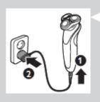
1 Insert the small plug into the appliance and put the adapter in the wall socket.
