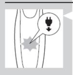
The appliance is equipped with an 'unplug for use' reminder. The 'unplug for use' starts to flash to remind you that you have to disconnect the appliance from the adapter before you can switch it on.
