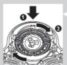
6 Place the retaining rings back onto the shaving heads and turn them clockwise.
