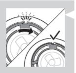
Each retaining ring has two recesses that fit exactly in the projections of the shaving head holder.Turn the ring clockwise until your hear 'click' and the ring is fixed.
