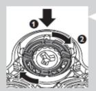
7 Place the retaining rings back onto the shaving head holder and turn them clockwise.
