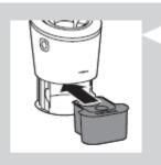
5 Place the new cleaning cartridge in the SmartClean system.
