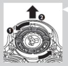
2 Turn the retaining rings anticlockwise and remove them.
