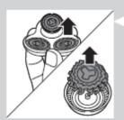
3 Remove the shaving heads from the shaving head holder. Each shaving head consists of a cutter and guard.
