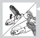
4 Take out the battery holder and cut the battery tags with a pair of cutting pliers.
