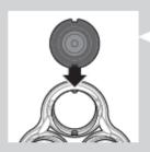
Note: Make sure the notches on both sides of the shaving heads fit exactly onto the projections in the shaving-head holder.
