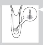
When the battery is almost empty, the bottom light flashes orange.
