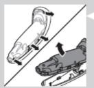
2 Bend the hooks aside and remove the power unit.
